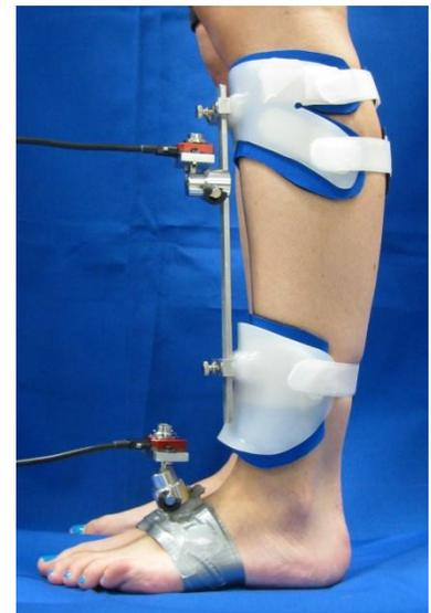
**Figure 3.** Tibia and Forefoot Cuffs with attached Inertial Measurement Units (IMUs).
