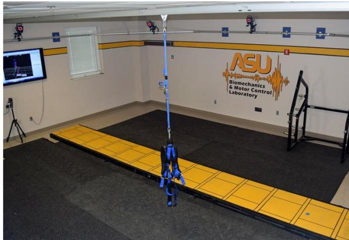
**Figure 1 - The Biomechanics and Motor Control Laboratory was refurbished and improved to handle data collection by installing a solo-step track and harness and reconfiguring the camera locations.**
