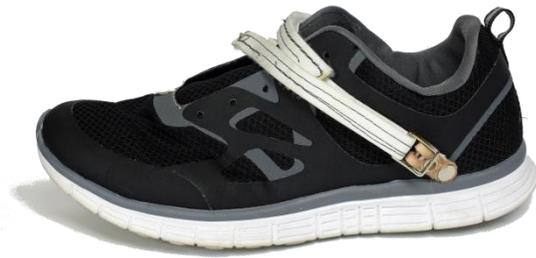
**Figure 6 - Shoes were acquired to control this variable across subjects. The shoes were modified to better fit the prosthetic feet and allow for quick removal to facilitate efficient data collection.**
